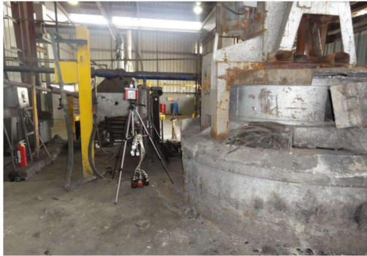
Figure 3. Area air sampling location 3 – sampling pumps were located between two kettles
