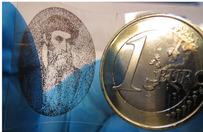
Figure 4. Johannes Gutenberg's portrait inkjet printed on a PET film by using the PdCu method.
