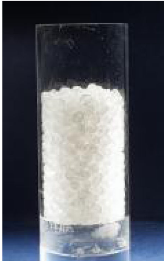
Figure 3. Bead phantom used to generate random background images. The phantom is filled with non-uniform polystyrene beads which are then stirred after each image to simulate object variability. Radioactive liquid occupies the negative space surrounding the beads.
