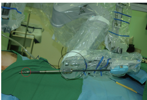
Figure 7 Parts of the ProGrasp forceps are showing; red circle indicates endowrist and black circle is external 3 rd joint of the ProGrasp forceps.
