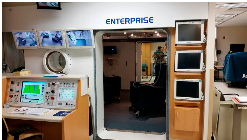
Figure 2. A multiplace hyperbaric/hypobaric chamber. Participants slept in a flat hospital bed placed in the chamber.
