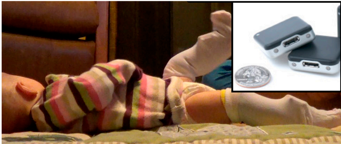
Figure 1. Three-month-old infant wearing sensors on the front of each ankle. Inset: Inertial sensors (Opals; APDM Inc., Portland, OR, USA) are synchronized, wireless, small and lightweight. They measure 48.4 \times 36.1 \times 13.4 mm (L \times W \times H) and weigh just under 22 g each. Opals are shown with a standard U.S. quarter for size reference.
