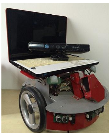
Figure 13. RGB-D SLAM system architecture based on Dr Robot X80.
