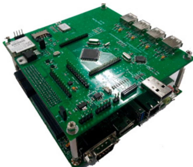
Figure 5. Prototype of the smart vehicular camera device based on NVIDIA Jetson board with the proposed extension board.
