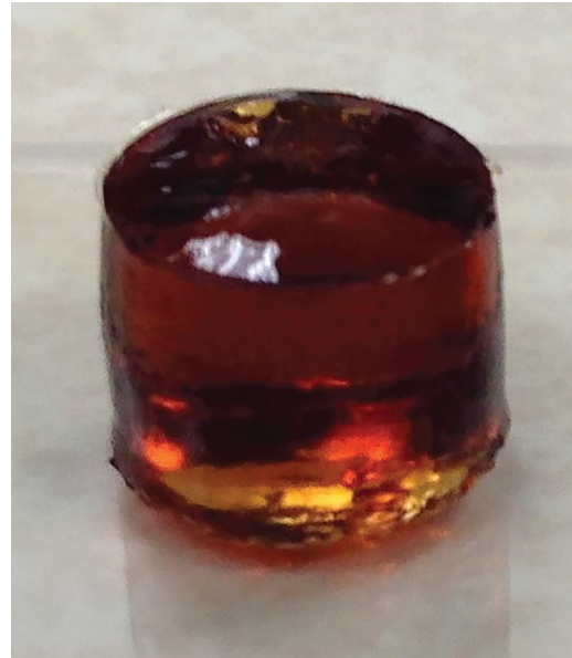
Fig. 4 Formed adhesive gel for compression testing
