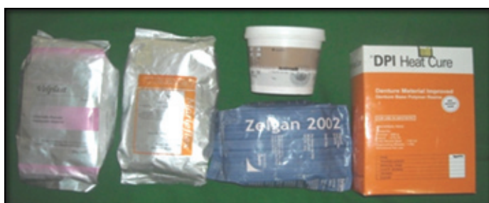
[Table/Fig-1]: Showing the materials used in the study -three brands of alginate-Velplast, Marieflex, Zelgan, type IV gypsum and heat activated autopolymerising resin
