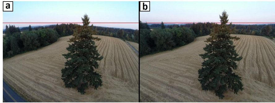
Fig 2. Removal of lens distortion. Demonstration of a. original, vs. b. OpenCV-calibrated lateral tree image obtained with a UAV-based GoPro camera at an above-ground altitude of 18 meters. Horizontal red line drawn to illustrate form of horizon in each version of the image.
