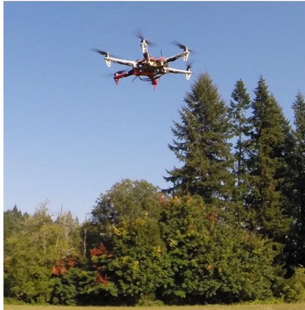
Fig 4. Custom built UAV hexacopter used to collect imagery data in this study.
