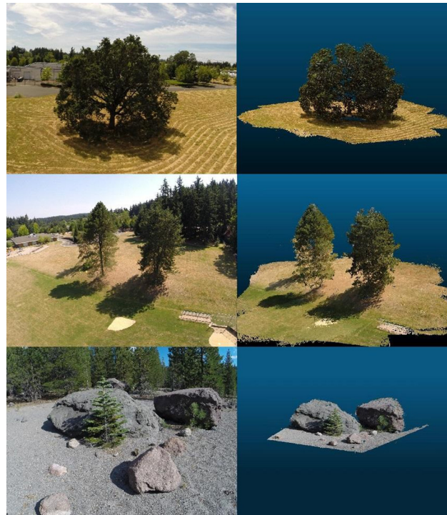
Fig 9. Illustration of comprehensive tree reconstructions (right column) and reference UAV-based images (left column).
