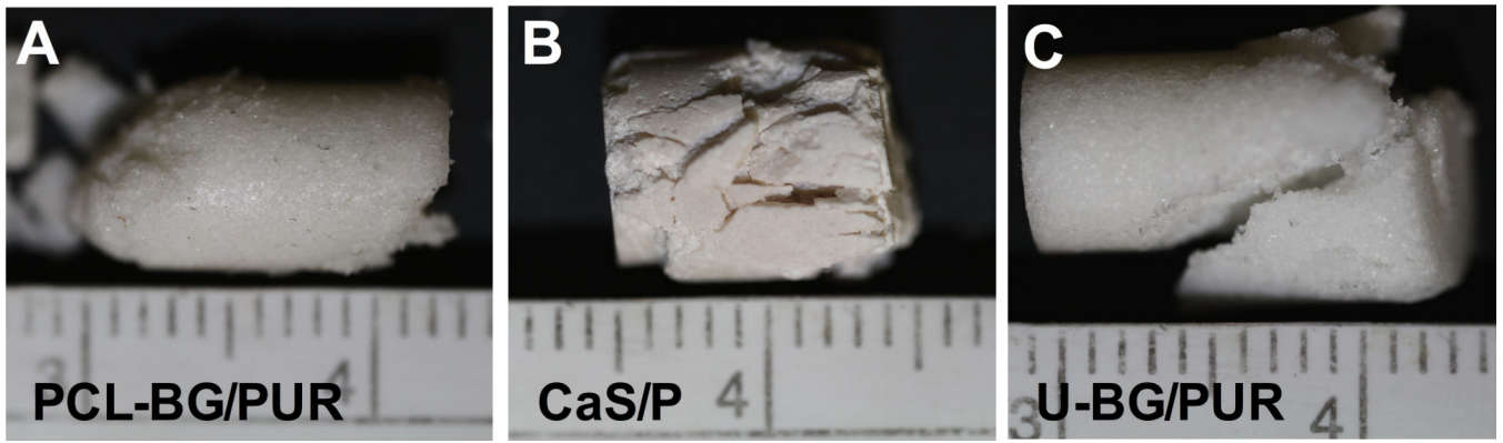
Figure 4. Macroscopic specimen failure. Images of specimens post-fatigue testing (strain= 5%): (A) PCL-BG/PUR, (B) CaS/P, and (C) U-BG/PUR. Centimeter ruler shown in images.
