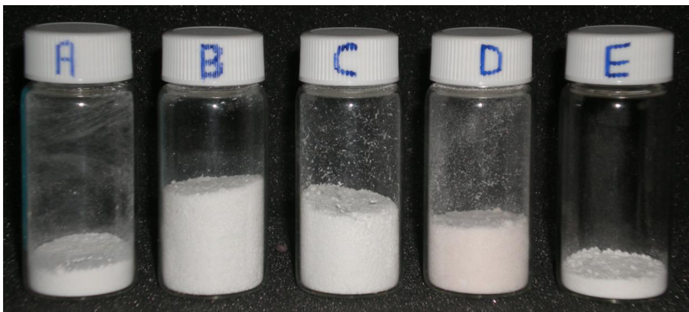
Fig. 4. Comparison in the density for the same mass between A) fluticasone powder as received, B) fluticasone nanoparticle agglomerates, C) Flu/Albu combination, D) albuterol nanoparticle agglomerates and E) albuterol powder as received.
