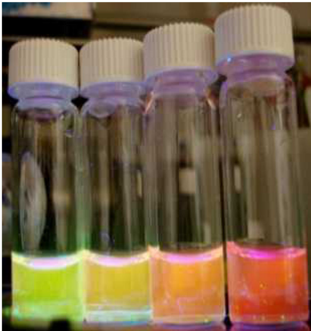
Fig. 3. Changes in emission color of the NC-SNARF sensor from left to right: pH = 6, 7, 8 and 9.
