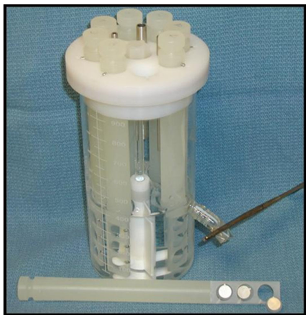
Fig. 1 The biofilm reactor is a device that incorporates eight polypropylene rods in a circular orientation inside a 1-L container; in the center of the aligned rods is a baffled stir bar.
