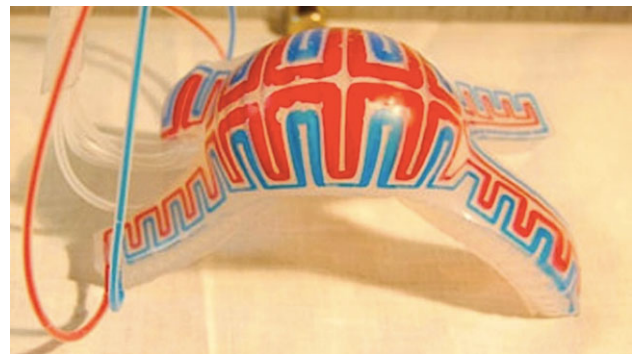
Figure 6. Cephalopods such as squid, octopuses, and cuttlefish use their ability to change colour to hide from predators. This soft robot uses simple microfluidic channels to camouflage its ‘skin’, hiding from detection in both the visible and infrared [23].
