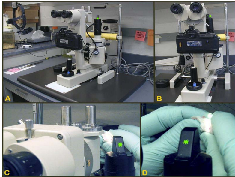
Figure 8. A–B: Slit lamp biomicroscope for the examination of the anterior segment (i.e. iris, cornea, lens) of the eye. C–D: Close-up of the light source (green asterisk) of slit-lamp in A–B .
