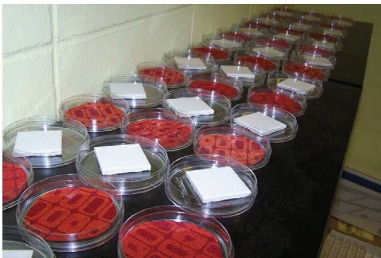
Figure 1. Both soft and hard substrates were treated with insecticides and stored uncovered for 3 months, then covered for 3 more months.
