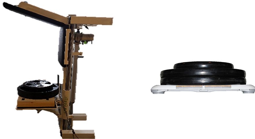
Fig 1. Still pictures of the calibration setup for the SID (left) and the WBB (right).
