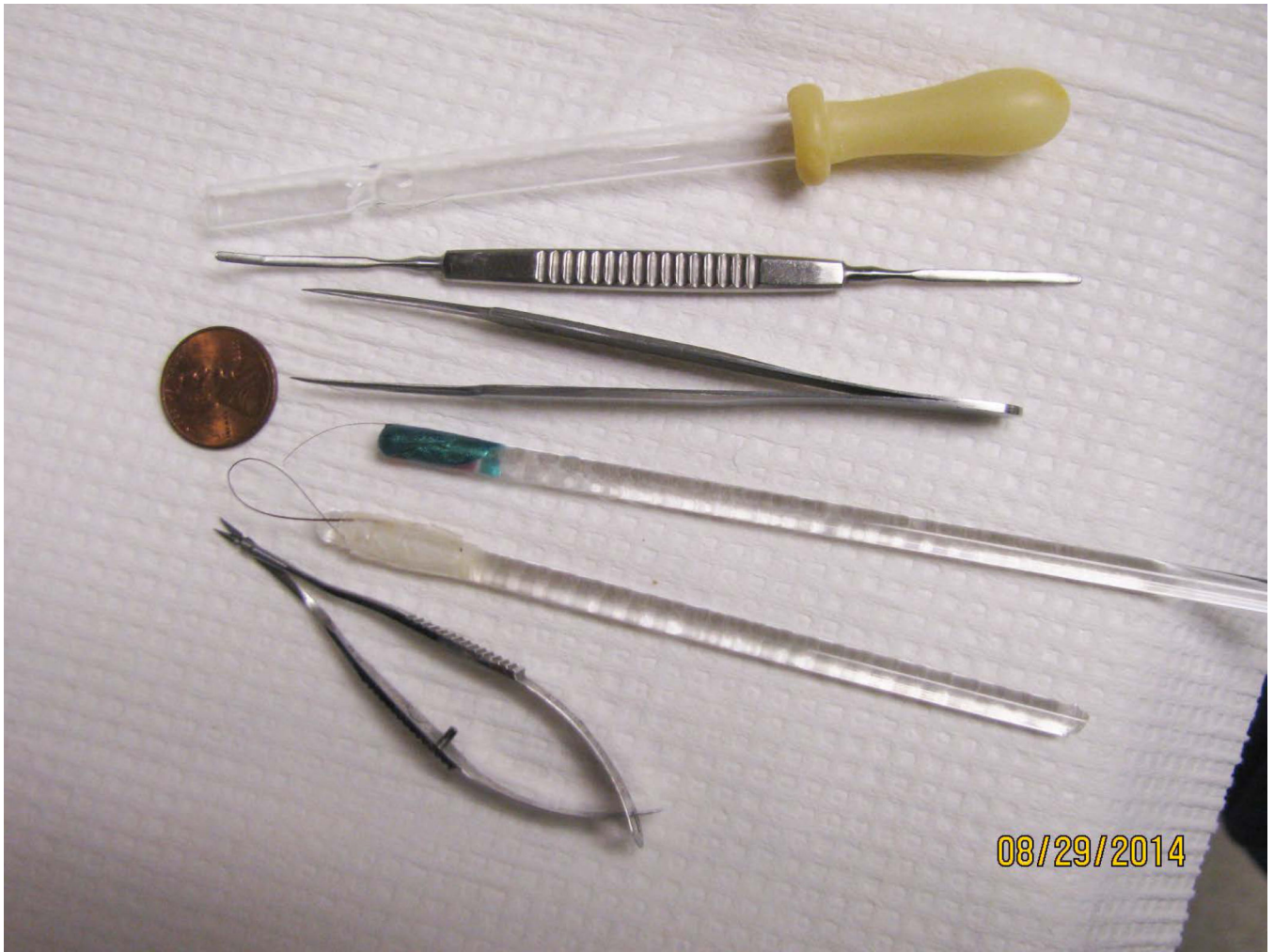
Fig 1. Tools used to isolate retinal vasculature in the elastase or trypsin digestion methods. Shown are an inverted pasteur pipette (used to pick up the fragile retina or vasculature), micro-spatula, toothed forceps, 2 single hair brushes, and Vannas micro-scissors. A penny is added for size comparison.
