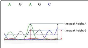
Fig. 1 The peak height G/A ratio was defined as the peak height A was devided by the peak height G
