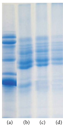
FIGURE 5: SDS-PAGE of protein patterns of SPI and SPI-dextran conjugates obtained by heat and TiO 2 photocatalysis. ((a) SPI; (b) control sample; (c) TP1; (d) TP2).
