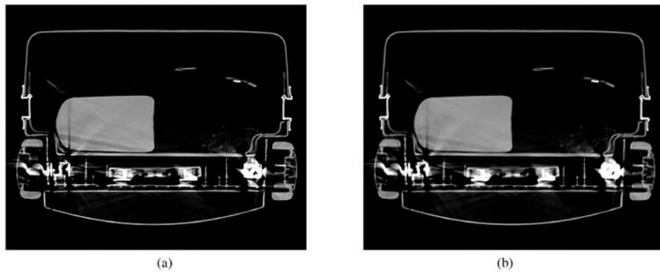
Fig. 2. DS1 reconstructions using minimum norm regularization: (a) SIRT-RWLS using \beta = 1.0 and (b) SIRT-RWLS using \beta = 5.0 . Image intensity levels truncated to 0-1800 MHU.
