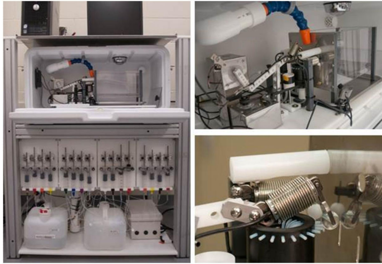
Figure 9. Photographs of the mouse version of the new gustometer. Reprinted from Spector AC, Blonde GD, Henderson RP, Treesukosol Y, Hendrick P, Newsome R, Fletcher FH, Tang T, Donaldson JA. (2015) A new gustometer for taste testing in rodents. Chem Senses , 40: 187–96 with permission.
