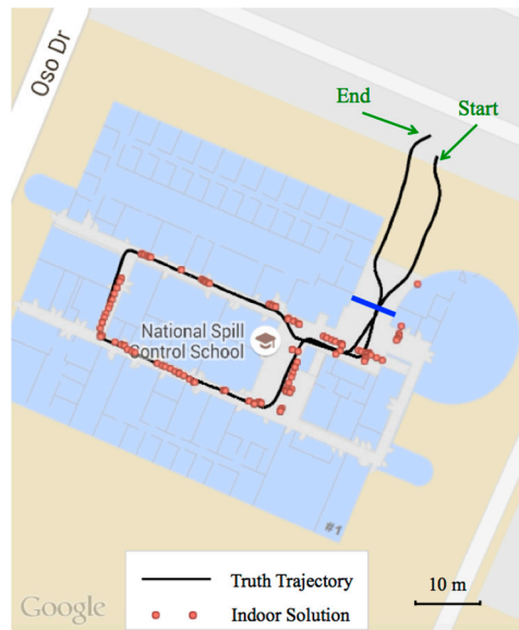
Figure 4. The trajectories of the indoor positioning solution with a Samsung Galaxy Note 3 smartphone and the ground truth generated by the NovAtel SPAN-IGM-S1 system.
