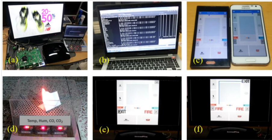
Figure 27. Demonstration of the use case scenario on a WoO service platform, which includes (a) smart gateway and sensors; (b) Application Server; (c) user interface; (d) fire occurrence and (e,f) signage.
