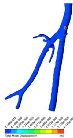
Figure 6 Mesh deformation contour plot of left CFA with DFA and SFA Plaques occurrence was modelled solely in left CFA (in red); area of mesh displacement indicates plaque formation
