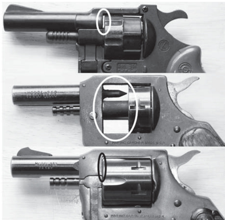
Figure 3. Side view of Kimar .22 starter pistol (top), H&R .32 starter pistol (middle), and H&R .32 revolver (bottom). Circled areas highlight the space between the cylinder and the barrel. In combination with a blocked barrel, the Kimar .22 and H&R .32 starter pistols have a significant gap between the cylinder and barrel, yielding a pathway for gasses to exhaust to the side. The H&R revolver has a very tight fit of the cylinder and the barrel, yielding negligible gap.
