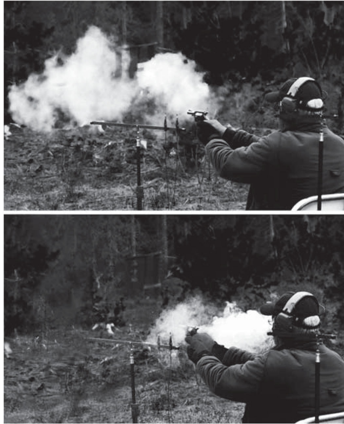
Figure 4. Picture of .32 H&R revolver (top panel) and .32 H&R starter pistol (bottom panel) both firing blank cartridges. The pattern of gas escape as evidenced by the black powder smoke is to the front for the open-barreled revolver and to the sides for the starter pistol. These images have been contrast-enhanced to increase visibility of the black powder smoke pattern.
