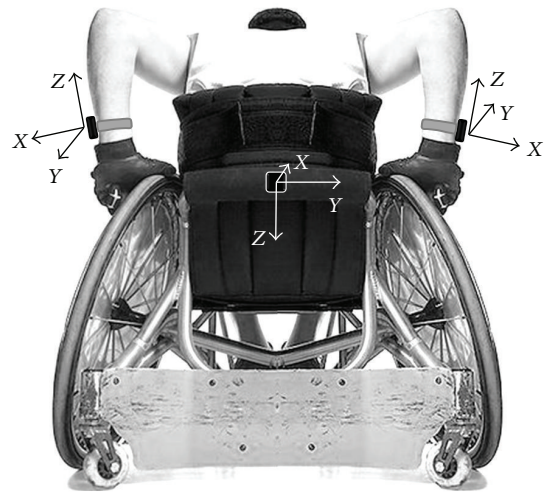
FIGURE 1: Wheelchair- and wrist-mounted IMUs with the relevant systems of reference.
