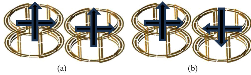
Fig. 2. Possible quadrature B_1 field arrangements (a) with the B_1 fields in the same direction. (b) with the B_1 fields in opposite directions. The arrangement on the left was chosen based on numerical simulations.
