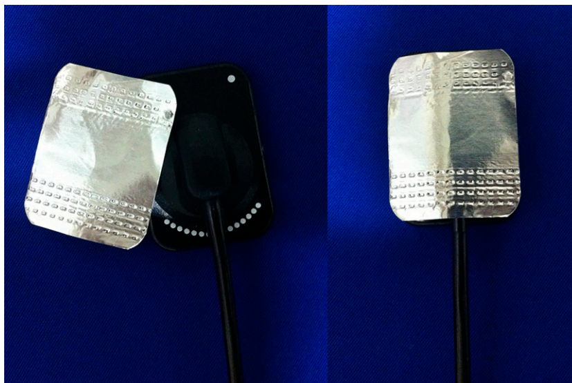
Figure 4 Image of the complementary metal oxide semiconductor (CMOS) digital periapical system (DIGORA ® Toto, Soredex ® , Tuusula, Finland) used and the location where the lead foil was placed.
