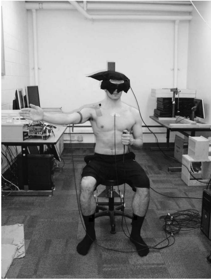
Figure 1. Experimental setup showing sensors, head-mounted display, and Kinesio Tape (Kinesio Precut, Albuquerque, NM).
