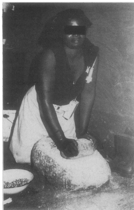
Figure 1 Transkei woman grinding maize in a poorly ventilated hut. The maize kernels (in the bowl) are ground between the oblong top rock and the large base rock. The personal dust sampler used in the study is strapped to the woman's waist and lapel.
