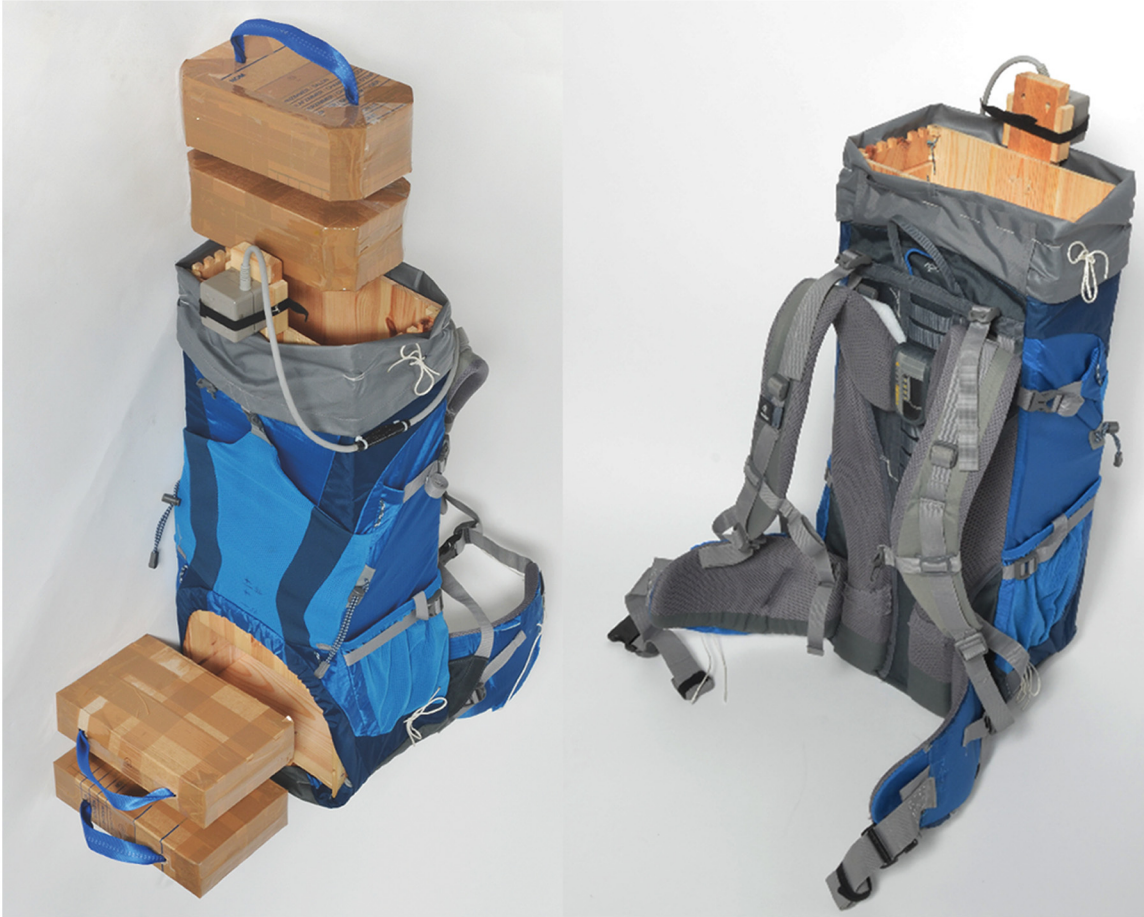
Fig 1. Modified load carriage system. The modular payload is shown on the left.
