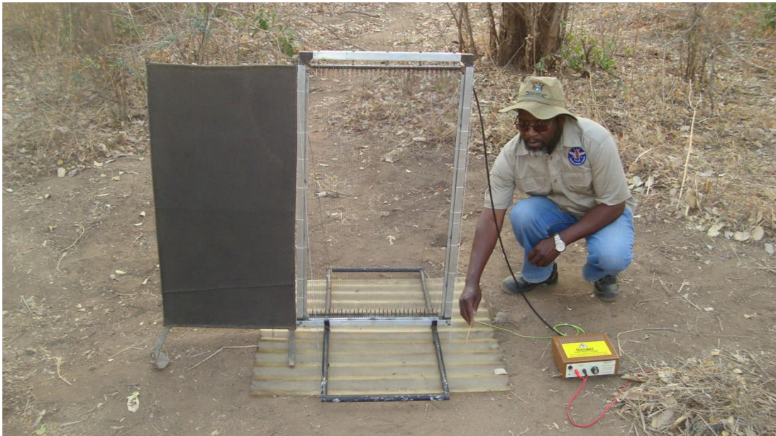
Fig 2. E-net by cloth. The yellow labelled box is the transformer, which was powered via the red leads from a battery hidden at the bottom right in a small pit covered by leaf litter. The black lead to the top of the E-net carried the high voltage output, and the yellow/green lead is the earthed return. A mirror image of this arrangement occurred 1.5m or 200m to the left, for the one-site or two-site methods, respectively.
