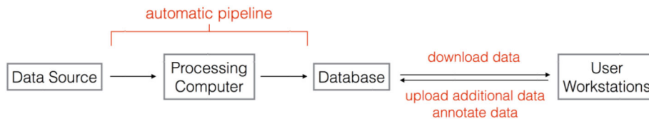
Figure 1. Workflow of the Caltech Tomography Database and Automatic Processing Pipeline This schematic shows the flow of data (arrows) through hardware elements (boxes) resulting from the indicated processes (red). Briefly, the Automatic Processing Pipeline collects tilt-series from a data source, either the collecting microscope (“real-time” mode) or a hard drive (“off-line” mode). Tomographic reconstructions, as well as key images and movies, are then generated by the processing computer, a basic workstation equipped with reconstruction and movie-making software. These automatically-generated files are then uploaded to the database, which consists of servers (web and MySQL) and a disk array. Individual users can browse the database, add annotations, download data to their personal computers, and/or upload additional data files. See Materials and Methods for detailed specifications.
