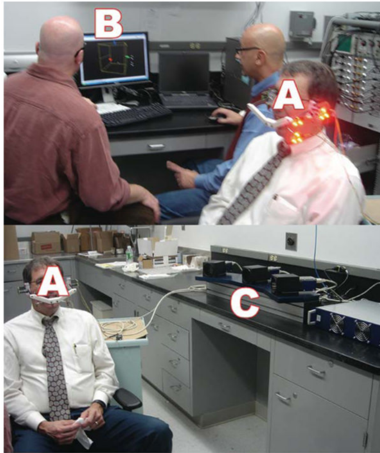
Figure 4. Opto-electronic tracking and capture of movement of the mandible in real-time. Three triangular target frames, carrying three non-collinear light emitting diodes (LEDs) each (A) are shown for the left side. The most posterior target frame is attached to the head reference system and occlusal registration appliance. The two anterior target frames defined maxillary and mandibular coordinate systems and were fixed temporarily to the vestibular surfaces of maxillary and mandibular canines and first premolars on one side by means of custom splints. The LEDs determined head- and mandible-related coordinate systems (B). The time-varying maxillary and mandibular LED positions were recorded by three linear cameras (C) with fixed geometry and resolution of better than 10\ \mu\text{m} at a sampling frequency of 200 Hz. Motion of the lower jaw was calculated relative to the head, thus, head motion was eliminated. Motion was viewed in real time during the experiments (B).
