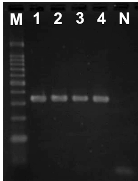
Fig. 2. Agarose gel electrophoresis of the products (339 bp) of Pentatrichomonas hominis species-specific PCR. M, 100-bp ladder; 1-4, DNA samples of cultures from trichomonad trophozoite-positive feces; N, water (negative control).
