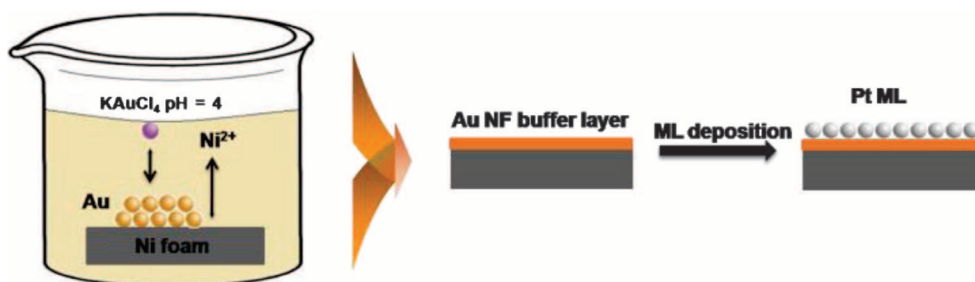
Fig. 1. Schematic illustration of the Pt monolayer fabrication process on Au-buffered Ni foam.
