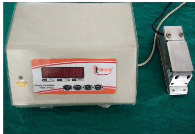
Fig. 1 Bite meter used for bite force evaluation
