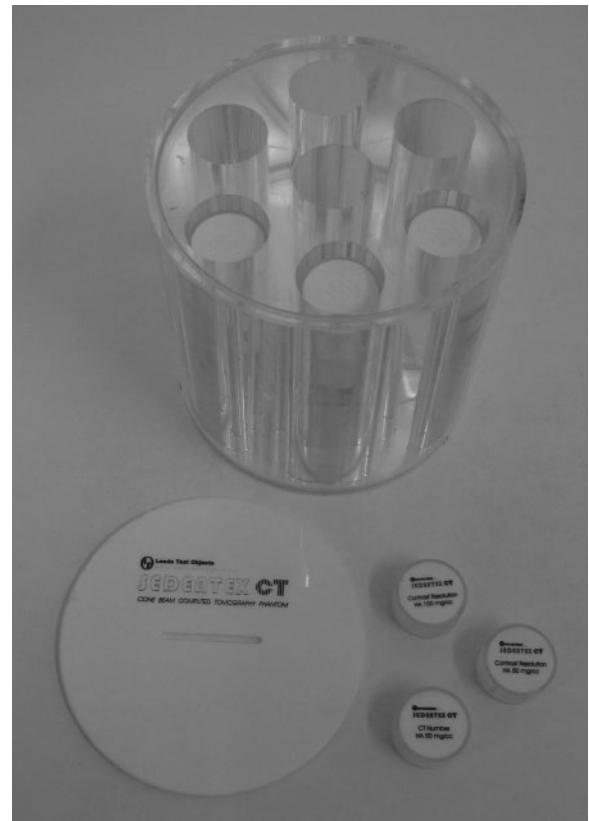
Figure 1. Customised polymethyl methacrylate phantom for the evaluation of grey values. The insert holder of 16 cm diameter is shown along with a selection of inserts of 3.5 cm diameter. In this study, six types of inserts were used containing materials of different density.
