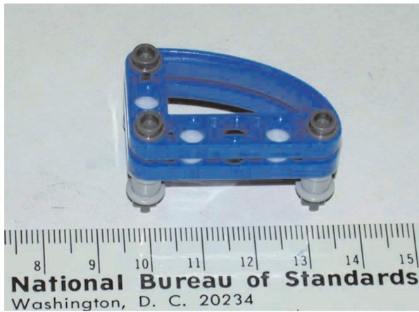
Fig. 1. A photograph of the assembled LEGO structure shown with PTFE spheres. The ruler is marked in cm.
