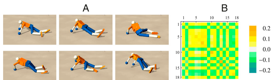
Fig. 2. Behavior exploration of the humanoid robot. (A) Crawling-like motion patterns when on the floor. (B) The corresponding controller matrix C reveals a definite structure. Note that the threshold dynamics was included here, which is an important factor for this highly organized behavior.
