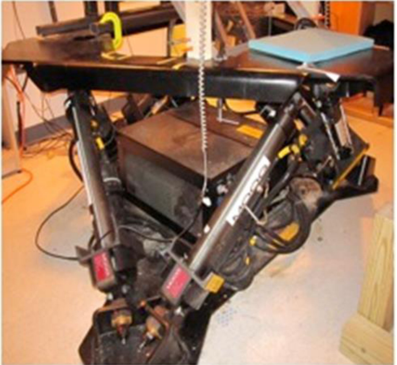
Fig 2. The system of hydraulic pistons guarantees wide range of motion of the MOOG platform.
