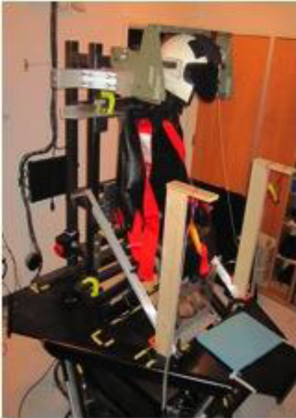
Fig 1. Chair on the mobile MOOG platform, adapted to immobilize the patient during testing
