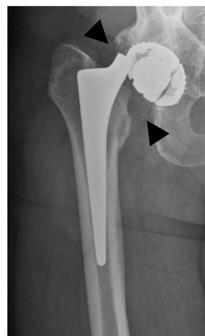
Fig. 29 AP radiograph. Cementless total hip arthroplasty. Proximal prosthetic/metallic fracture through the neck of the femoral implant (arrowheads)
