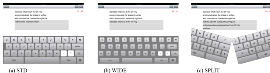
Fig 2. The three different designs of virtual keyboard evaluated. (a) STD design, the default layout provided in the tablet's operation system. (b) WIDE design, the layout with broaden horizontal between-key spacing. (c) SPLIT design, the layout formed by two angled half keyboards
