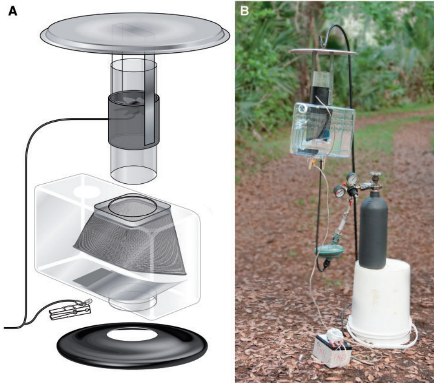
Fig. 2. Automated updraft carbon-dioxide baited light trap. Panel A: Diagram of trap. Panel B: Trap in field setting. See Materials and Methods for complete description.
