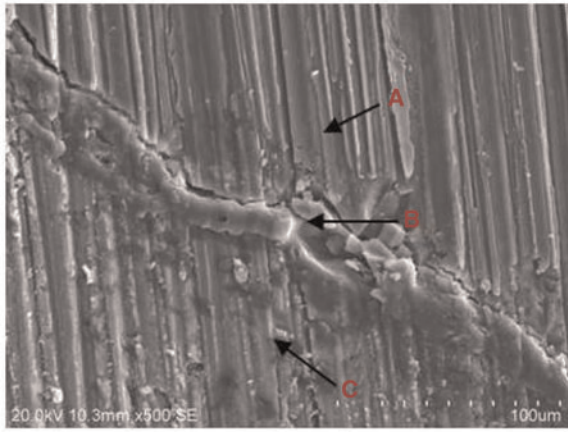
Figure 10. SEM image of the MAO-coated pure Mg implant and the surrounding bone tissues after 4 weeks' implantation.
