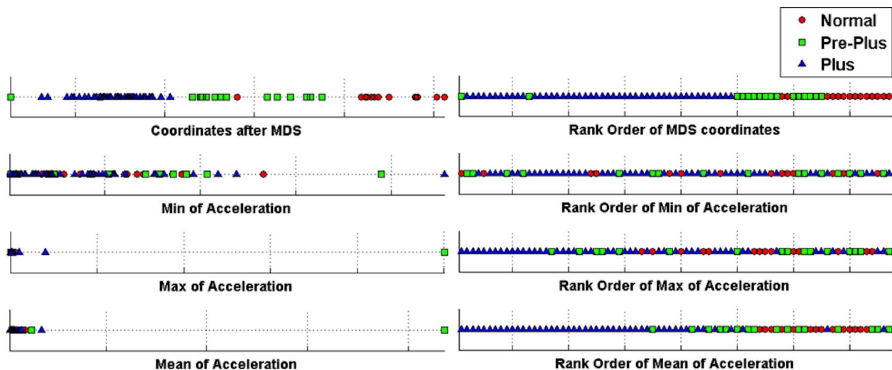
Figure 5. Results of nonlinear dimensionality reduction by applying MDS on GMM-based distance (top) and regular statistics (minimum, maximum, mean) of the acceleration feature. Left shows the 1-D MDS coordinates and the minimum, maximum, and mean of acceleration respectively. Right shows the rank of image when it is ordered based on corresponding MDS coordinate or acceleration statistic.
