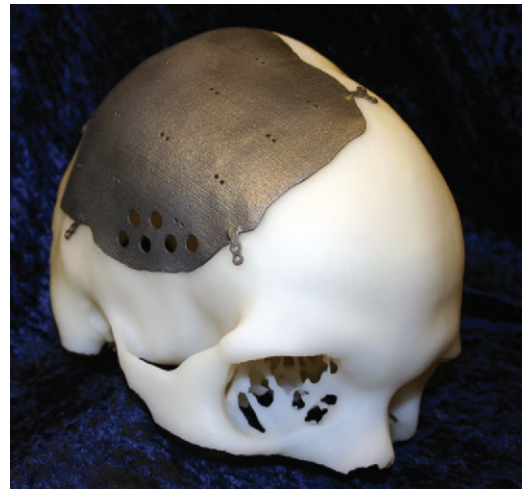
Figure 9. Three-dimensional printed model created for a patient scheduled for placement of a titanium cranial plate. A model of the patient's skull was printed with stereolithography. The plate (Ti6AlV4 alloy) was 3D printed with electron-beam technology. This type of surgical planning enables a precise, patient-specific intervention that decreases the time required for the intervention and the risk for peri- and postoperative complications.
